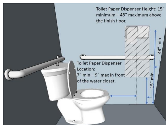
Figure 2.15 Toilet Paper Dispenser
