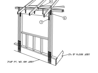
TYP. HEADER & CONNECTORS FOR 3 OPENINGS AT EXT. BEARING WALLS 52
