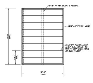
FLOOR FRAMING PLAN SCALE 1/8" = 1'-0"
