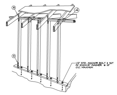
TYPICAL EXT. WD. FRAME BEARING WALL CONNECTIONS & STRAPPING (52)
