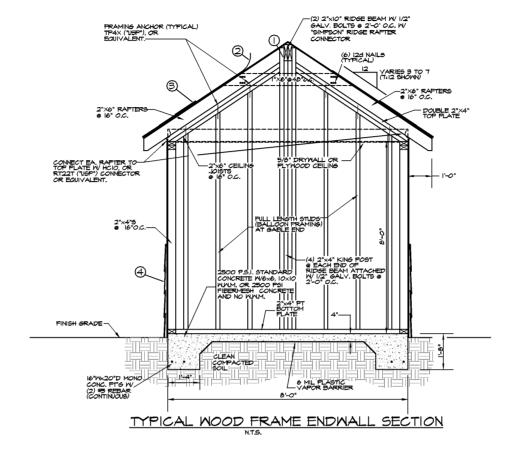
MHEN BLDG. IS LOCATED WITHIN A FEMA FLOOD ZONE AREA, HYDROSTATIC VENTING IS REQ'D. HYDROSTATIC VENTING SHALL BE SO ARRANGED TO PERMIT THE AUTOMATIC PASSAGE OF STORMWATER. ALL VENTING SHALL BE LOCATED A MAXIMILM OF I'-O' ABOVE F.F. I SO, IN, OF VENTING SHALL BE REQ'D, FOR EA. SQ. FT. OF FLOOR AREA.
