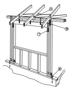
TYP. HEADER & CONNECTORS FOR 3 OPENINGS AT EXT. BEARING WALLS
