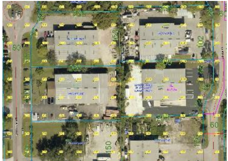
Figure 13. Screenshot of GIS application developed to check parcel elevation; Lee County GIS
