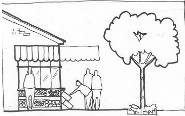
Figure 5: The utilization of flat canopies is discouraged except in circumstances where it is accompanied by a valance
