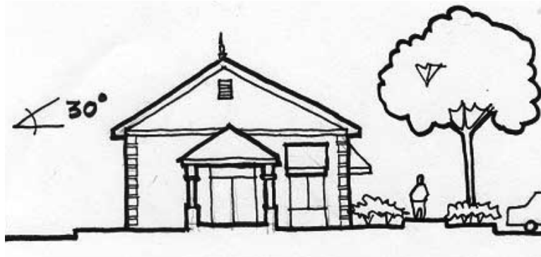
Figure 1: Buildings with less than 5,000 square feet must be designed with minimum 30° pitch roof
