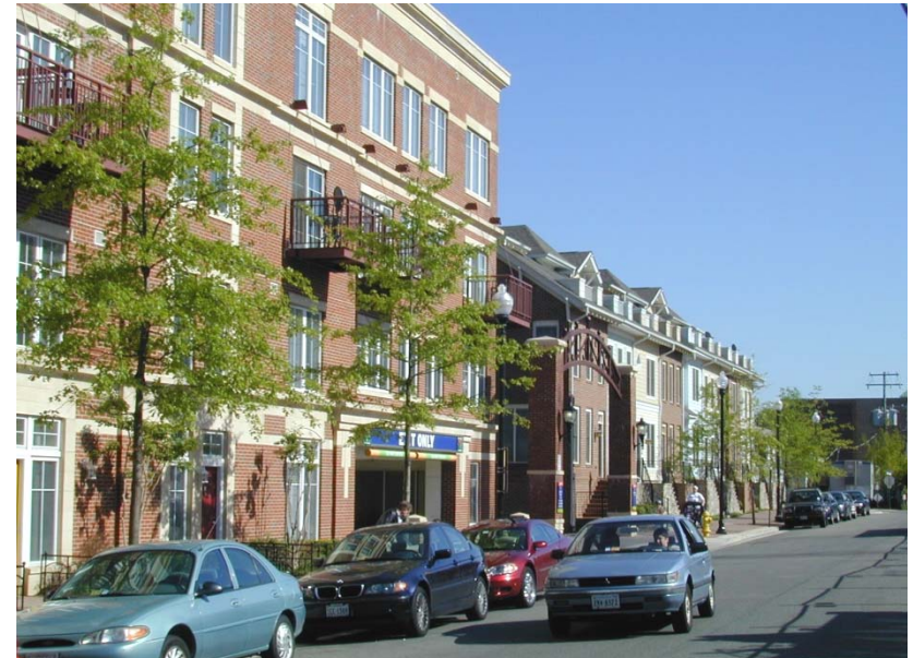
Building heights should step down along edges shared with established residential neighborhoods. In this example, townhomes are used to provide a more gradual transition in height between a mixed-use center and an adjacent single-family neighborhood.
