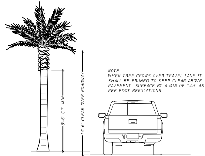
A VERTICAL CLEARANCE FOR PALMS 1/4" = 1'-0" P-BU-11
