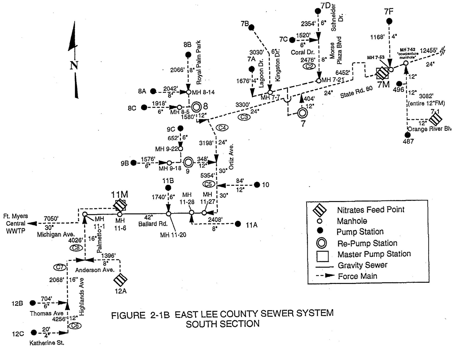
FIGURE 2-1B EAST LEE COUNTY SEWER SYSTEM SOUTH SECTION
