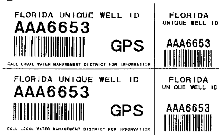
Figure V-8. Florida Unique Well Identification (FLUWID) Tag
