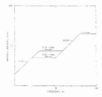
In actuality, since the USBM "Z" curve was developed for large scale mining operations, it could be followed as the limit for vibration without causing damage. But, humans are extremely receptive to vibration, and if this curve were followed, there would likely be many more complaints.
