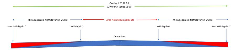
"AC asphalt roads shall be fade milled with a single pass on each side of the roadway from 0 on the centerline side and a 1" on low side or at a depth not to damage the existing base."
