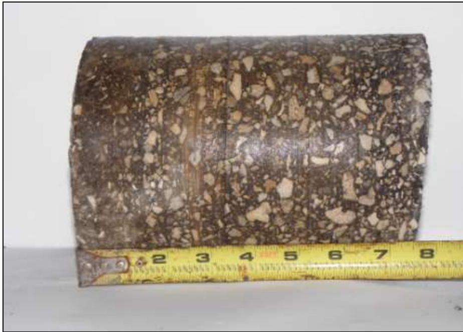
ASPHALT CORE C-1
