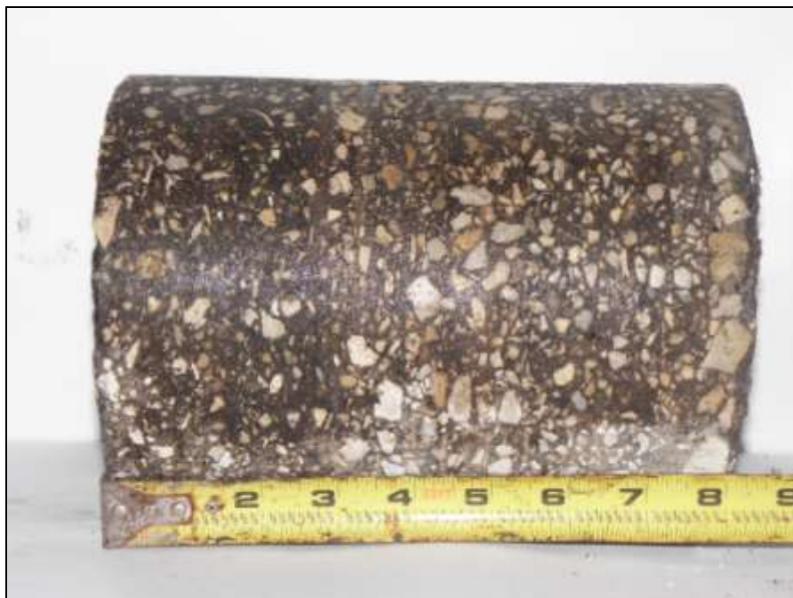
ASPHALT CORE C-6
