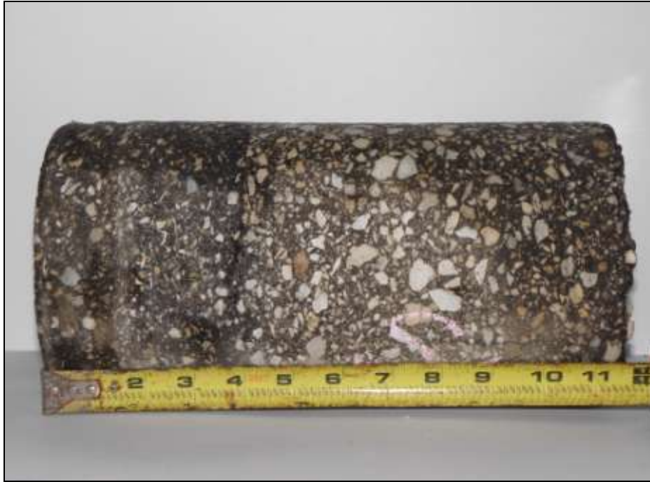
ASPHALT CORE C-1
