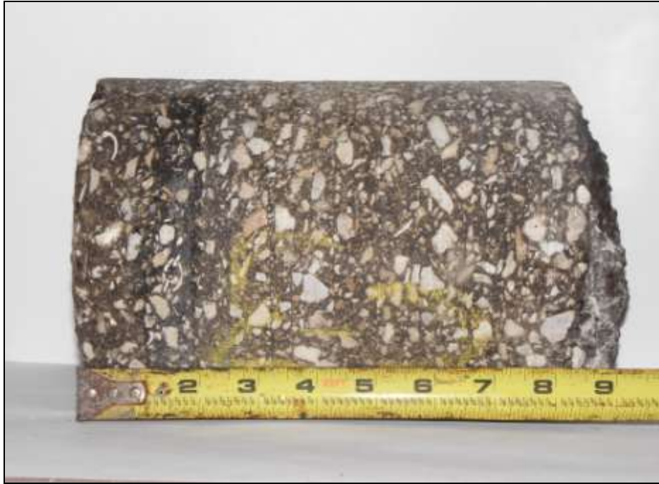
ASPHALT CORE C-3
