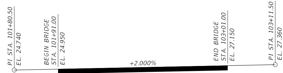
PROFILE GRADE DATA - ALONG Q BRIDGE
