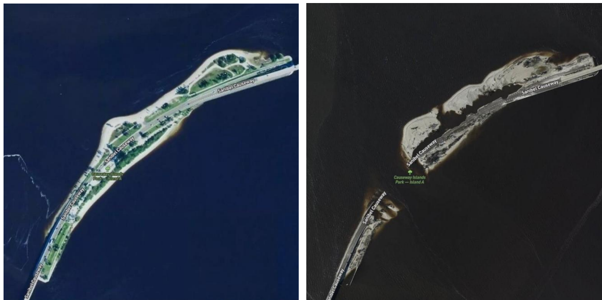
Figure 36 - Before and after imagery of a portion of the Sanibel Causeway, showing the damage of Hurricane Ian 129
