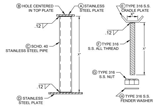
X" LENGTH VARIES DEPENDING ON OBJECT BEING SUPPORTED SEE TABLE THIS SHEET FOR DIMENSIONS A THRU H
