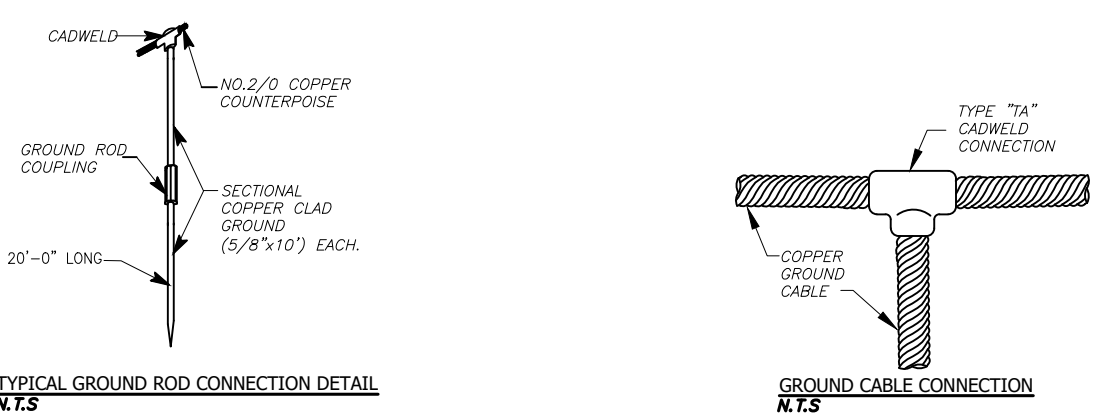
TYPICAL GROUND ROD CONNECTION DETAIL N.T.S.
